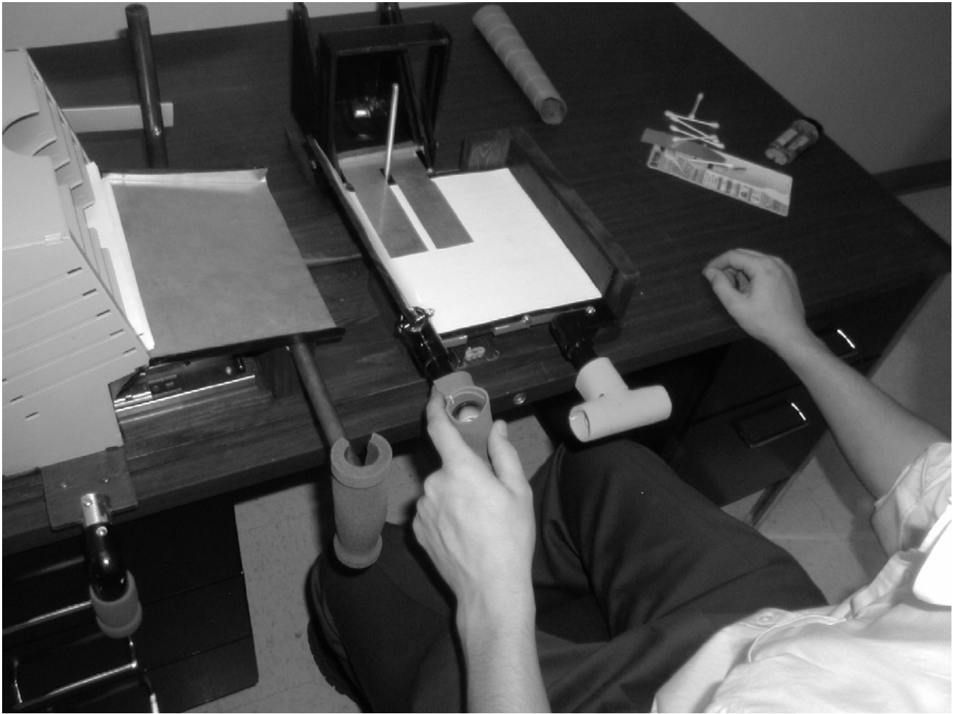
Figure 7.16. The Paper Management System, Shown Starting the First Fold
